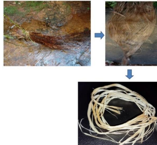
Figure 1: Process of preparation of Helicteres isora fiber
